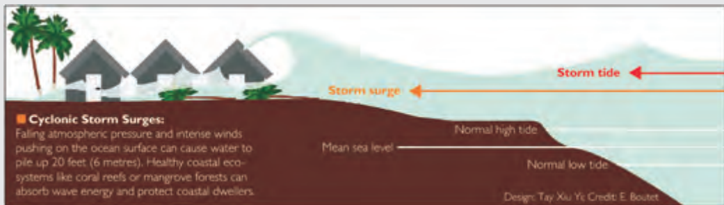
Figure 6.22: The most severe storm surges occur as a result of tropical cyclones – they are particularly severe when they occur during the time of a high tide.
